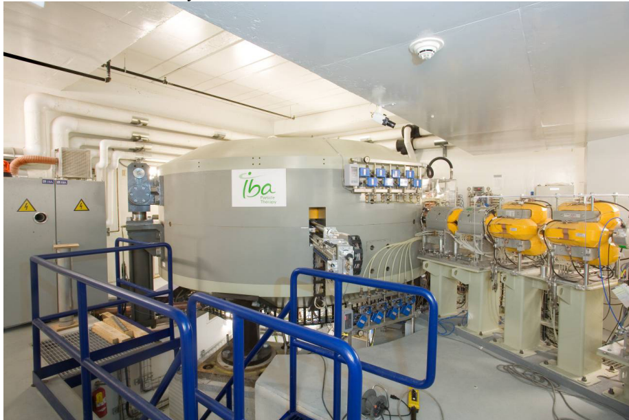
Figure 2. IBA 230 MeV resistive cyclotron for proton therapy
