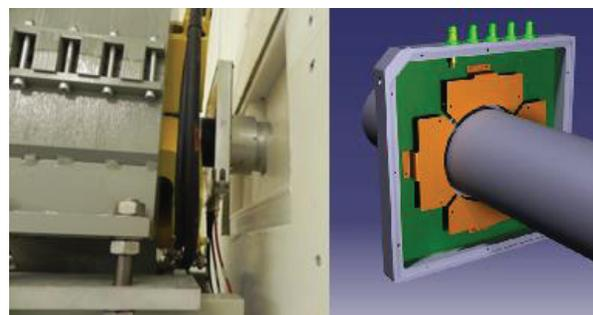
Figure 3: On the right, BLM installed between the wall and a quadrupole. On the left, the designed BLM.
