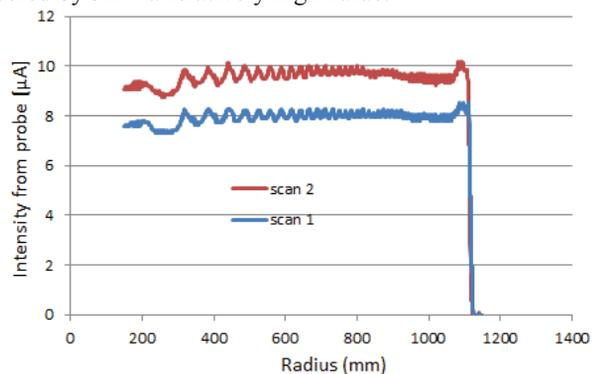
Figure 2: Intensity radial scan inside the cyclotron performed with the probe.
