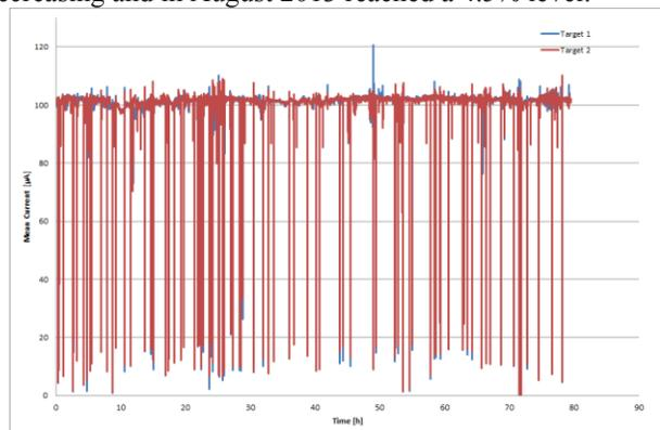
Figure 1: 80 hours of a dual-mode run at the intensity of 101.2  $\mu\text{A}$  on each beamline.
