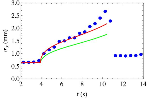
Figure 2: Experimental and computed horizontal beam width  $\sigma_x$  of a  $^{12}\text{C}^{6+}$  ion beam ( $28\mu\text{A}$ ) as a function of time during deceleration. Deceleration starts at  $t=4$  s. Two cooling steps were applied at  $t=0$  s and  $t=11$  s. The final energy is 9.7 MeV. The red and green lines are computed beam width with equation (8) for  $\kappa = 3.25$  and  $\kappa = 3$ , respectively.
