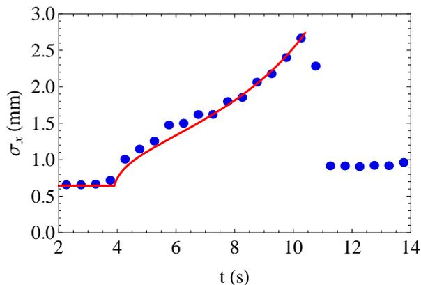
Figure 3: Development of  $\sigma_x$  of a  $^{12}\text{C}^{6+}$  ion beam ( $I=28 \mu\text{A}$ ) as a function of time during deceleration. Computed  $\sigma_x$  for  $\kappa = 3$  is shown as red line.
