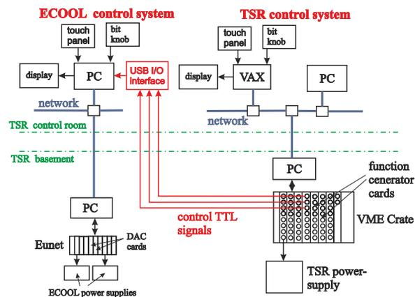
Figure 7: Schematic drawing of the TSR and ECOOL control system modification to enable electron cooling at various energies in the deceleration cycle.
