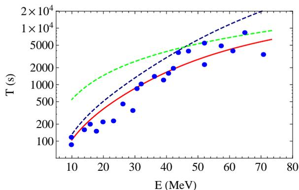
Figure 6: Measured lifetime of the  $^{12}\text{C}^{6+}$  beam for different energies. The green dashed line is the lifetime taken into account multiple scattering, whereas the blue dashed line represents the electron capture lifetime. The red solid line is the total lifetime calculated for  $p=7 \cdot 10^{-11}$  mbar.
