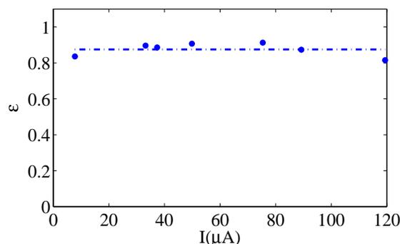
Figure 5: Measured deceleration efficiency as a function of the injected ion intensity.
