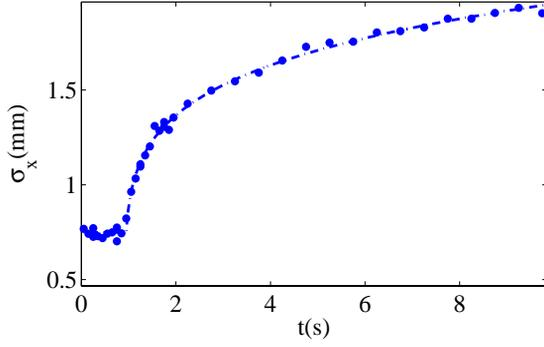
Figure 1: Measured horizontal beam width  $\sigma_x$  of a  $^{12}\text{C}^{6+}$  bunched ion beam (73.3 MeV,  $50\mu\text{A}$ ) as a function of time after 1.5 s. The dashed line through the data is a fit using equation 4 where  $\gamma$  is the fit parameter.
