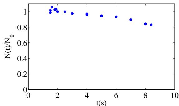
Figure 4: Measured number of particles  $N(t)$ , normalized to the injected particle number  $N_0$ , during deceleration of a  $^{12}\text{C}^{6+}$  ion beam from  $E=73.3$  MeV to  $E=9.7$  MeV. Deceleration starts at  $t=1.5$  s. At  $t=8.5$  s the final energy was reached.
