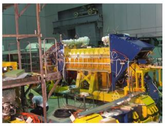
Figure 2: Assembling the 2 MeV electron cooler at BINP.
