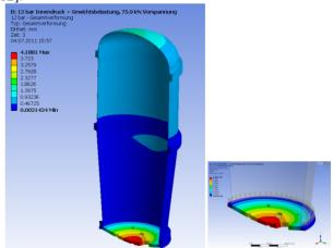
Figure 5: Mechanical stresses and deformations of the high voltage vessel.
