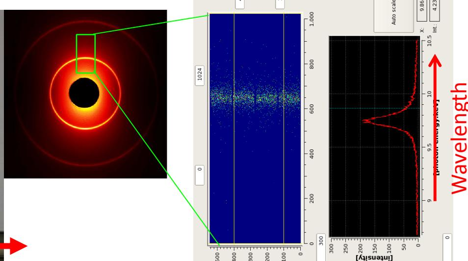
Wavelengths are calculated from positions of Debye-Scherrer rings on MPCCD.
