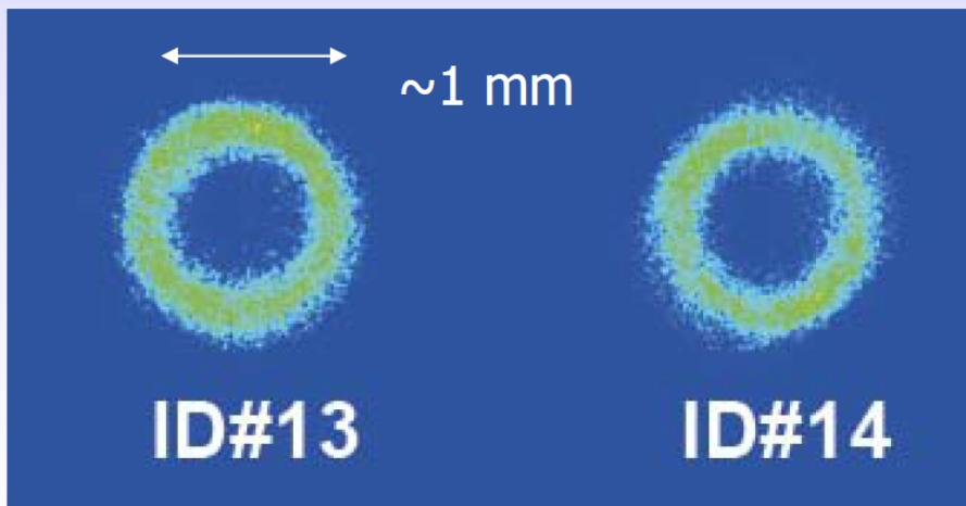
Straightness of electron beam over multiple segments of undulators
