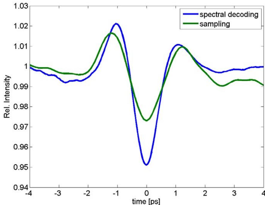
Spectral decoding laser modulation: 7 %
