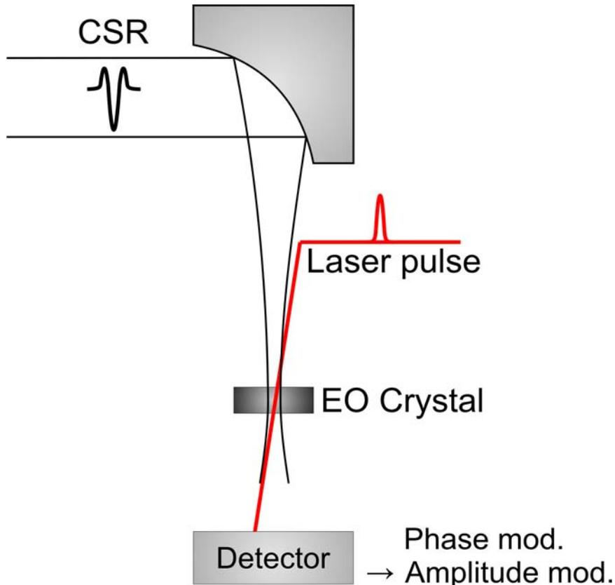
Synchronized Ytterbium fiber laser is modulated by Coherent Synchrotron Radiation ( $E_{\text{THZ}}$ ) in EO crystal (GaP, ZnTe)
