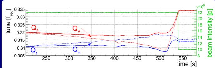
Coupling induced crossing of unperturbed tunes (dashed line) and eventually third-order resonance crossing of the vertical eigen-mode (solid line) leading to particle loss → fixed in the next squeeze iteration
