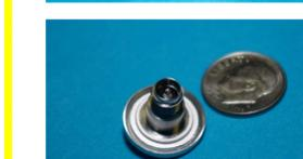
Button head is simple rod of diameter of 1.8mm
