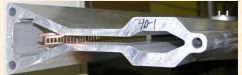
Fig. 6: Flexible BeCu RF shielding with 50% of open space inside of the multipole vacuum chamber. The thickness of the RF shielding is 0.25mm.
