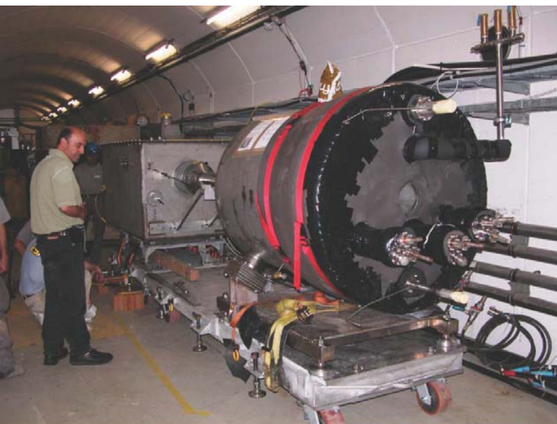
15-T solenoid and Hg jet installed in TT2A tunnel at CERN
