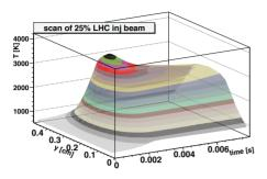
Figure 8: Distribution of wire temperature during a scan of LHC injection beam with 25% of the nominal intensity.
