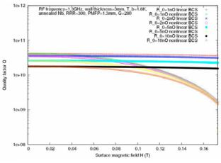
Figure 26: Variation of the cavity Q with RF surface magnetic field for residual resistance between 1 n $\Omega$  and 10 n $\Omega$ . In each case Q vs H curves are given for BCS and nonlinear BCS cases (in color).
