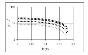
Figure 9: Variation of quality factor with magnetic field for residual resistances  $R_0 = 3 \text{ n}\Omega$  ( $\blacklozenge$ ),  $5 \text{ n}\Omega$  ( $\blacksquare$ ),  $10 \text{ n}\Omega$  ( $\blacktriangle$ ), and  $20 \text{ n}\Omega$  ( $\times$ ).
