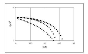
Figure 17: Variation of quality factor with magnetic field for thermal conductances of unannealed niobium ( $\blacklozenge$ ), annealed niobium ( $\blacksquare$ ), and nucleate boiling helium ( $\blacktriangle$ ).
