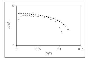
Figure 21: Measurement of Q as a function B for a 3.9 GHz TESLA cavity ( $\Box$ ) [4] compared with the results of a numerical simulation with matching cavity parameters ( $\blacklozenge$ ).
