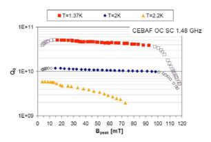
Figure 22: Measurements of Q vs B on a CEBAF cavity by Ciovati [6]. The T = 2.2 K curve (in yellow) is in the nucleate boiling regime and clearly shows a more linear than quadratic dependence of Q on B. (c.f. Figure 17.)
