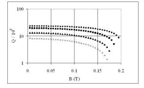
Figure 13: Variation of quality factor with magnetic field for bath temperatures  $T_b = 1.4 \text{ K} (\blacklozenge), 1.6 \text{ K} (\blacksquare), 1.8 \text{ K} (\blacktriangle),$  and 2.0 K (×).
