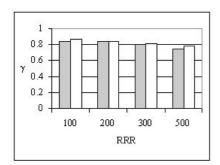
Figure 12: Medium field Q-slope values for varying residual resistivity ratio *RRR*, calculated numerically (shaded) and from Halbritter's approximate formula (unshaded).
