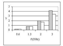
Figure 6: Medium field Q-slope values for varying RF frequency f, calculated numerically (shaded) and from Halbritter's approximate formula (unshaded).
