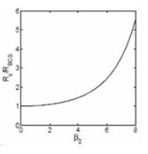
Figure 23: Increase of BCS resistance due to pair-breaking at high supercurrent density  $\beta_0$  [18].
