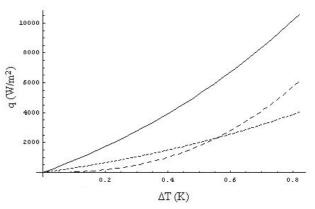
Figure 4: Thermal conductance across Nb-LHe interface as a function of temperature difference for annealed niobium (solid), unannealed niobium (short dashed), and nucleate boiling (long dashed).
