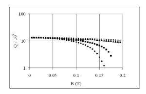
Figure 15: Variation of quality factor with magnetic field for phonon mean free paths  $l = 0.05 \text{ mm} (\blacklozenge), 0.1 \text{ mm} (\blacksquare), 0.5 \text{ mm} (\blacktriangle), 1.0 \text{ mm} (\times), and 5.0 \text{ mm} (+).$
