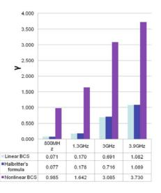
Figure 30: Gamma values for BCS and nonlinear BCS for various phonon mean free paths.
