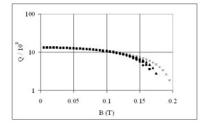
Figure 11: Variation of quality factor with magnetic field for residual resistivity ratios  $RRR = 100 (\diamondsuit), 200 (\blacksquare), 300 (\blacktriangle), and 500 (×).$
