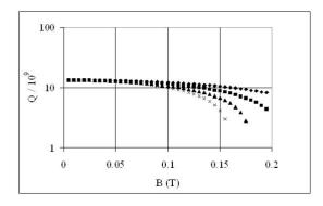
Figure 7: Variation of quality factor with magnetic field for wall thicknesses  $d = 1 \text{ mm} (\blacklozenge), 2 \text{ mm} (\blacksquare), 3 \text{ mm} (\blacktriangle)$ , and  $4 \text{ mm} (\times)$ .
