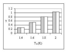
Figure 14: Medium field Q-slope values for varying bath temperature  $T_b$ , calculated numerically (shaded) and from Halbritter's approximate formula (unshaded).
