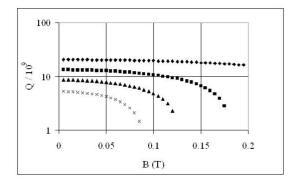
Figure 5: Variation of quality factor with magnetic field for RF frequencies f = 0.6 GHZ ( $\blacklozenge$ ), 1.3 GHz ( $\blacksquare$ ), 2.0 GHz ( $\bigstar$ ), and 3.0 GHz ( $\times$ ).
