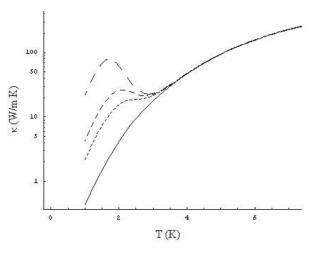
Figure 2: Thermal conductivity versus temperature for RRR = 300 and l = 0.1 mm (solid), 0.5 mm (short dashed), 1.0 mm (medium dashed), and 5.0 mm (long dashed).
