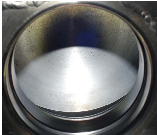
Figure 2: Damage of the central part of LIA-2 cathode by tantalum drops from the target. View on the cathode through the anode aperture.
