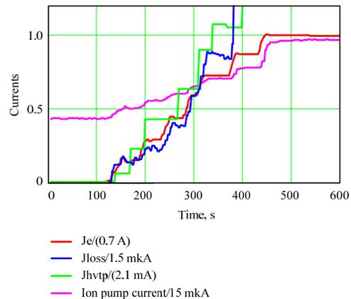
Figure 12: Measuring efficiency of collector capture at 30 keV.
