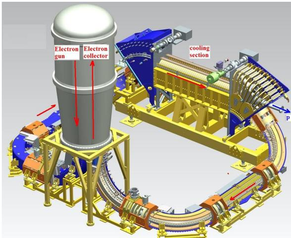
Figure 2: Sketch of 2 MV cooler for COSY.
