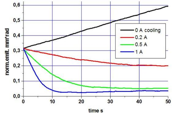
Figure 1: Cooling of 2 GeV proton beam .
