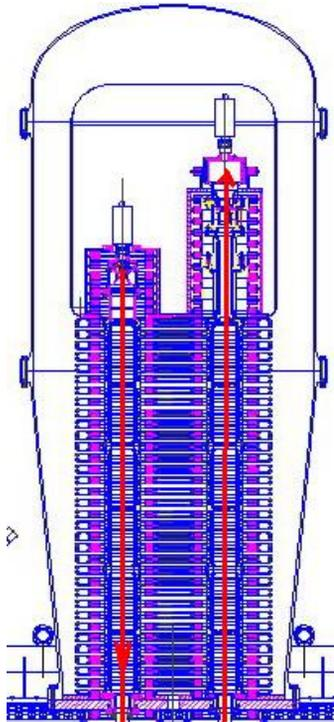
Figure 3: The high voltage tank of the cooler.
