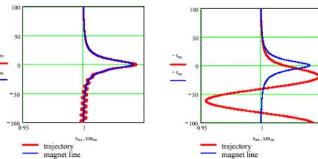
Figure 9: Passing of 10% variation of magnetic field by 0.2 MeV and 1MeV electron.
