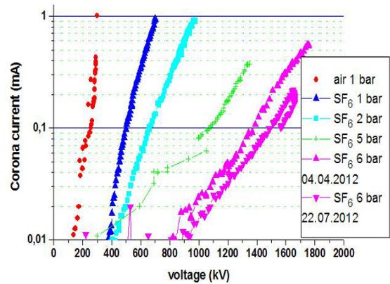
Figure 4: Corona current versus voltage for different SF<sub>6</sub> pressures.
