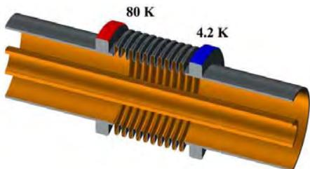
Figure 2: Model of a regular cold bellows
