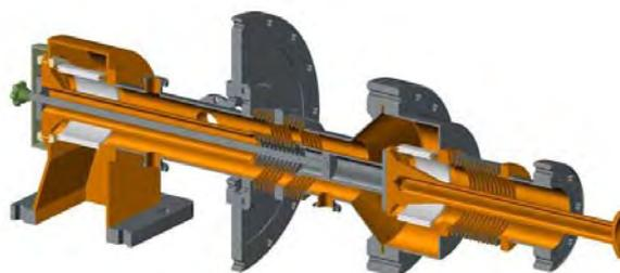
Figure 1: Input coupler for the ERL injector
