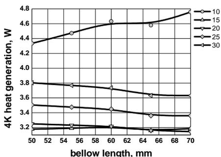
Figure3: Dependences of heat generation wattage on bellows length
