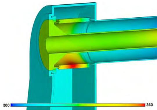
Figure 8: Temperature map of waveguide-to-coaxial transition
