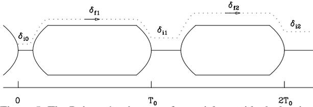
Figure 5: The Poincaré trajectory of a particle outside the barrier bucket with the left barrier pulse moving to the right.
