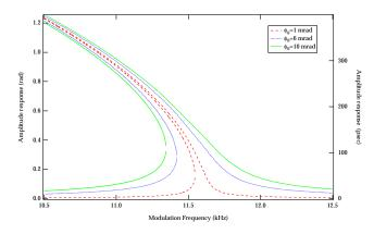
Figure 5: Response of driven longitudinal oscillations for 3 excitation amplitudes. The nominal synchrotron frequency is 11.6 kHz.
