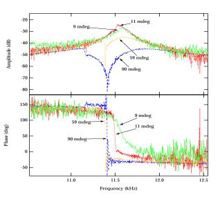
Figure 1: Amplitude and phase of longitudinal beam transfer functions for increasing frequency sweeps as a function of drive amplitude.
