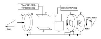
Figure 2: Schematic diagram of the streak camera in synchroscan mode with dual sweep. A: phothcathode, B: accel. mesh, C: vert. deflection electrode, D: horz. defl. electrode, E: microchannel plate F: phosphor screen, G: CCD camera.
