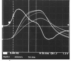
Figure 4—JBdl for Various Resistivity Beampipe Coatings. Beampipe I.D. 60.3mm with a) infinite  $\Omega/\Box$  ( $\tau_p=0$ ), b) 1.941 $\Omega/\Box$  ( $\tau_p=9.8$ ns), c) 0.572 $\Omega/\Box$  ( $\tau_p=33.1$ ns), and d) 0.180 $\Omega/\Box$  ( $\tau_p=105.2$ ns) coating resistivities.
