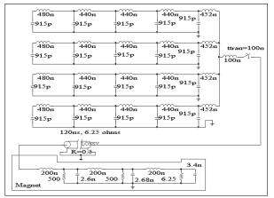
Figure 2—Pinger System Schematic used in Circuit Simulations
