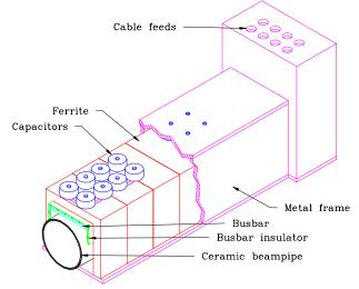
Figure 1—Quasi Traveling-Wave Pinger Magnet Geometry. Load not shown for clarity.
