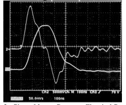
Figure 3—Pinger Magnet Prototype Electrical Response. Signals are a) direct B-dot signal and b) software integrated [Bdl (pulse).
