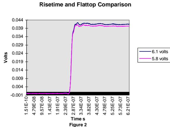
The data from the first set of measurements shows an ability to measure voltage changes to better than 2%. This is more a test of relative change rather than a measure of absolute field value. Since the only way to get absolute values is to DC test the ferrite and trace out the characteristic B-H curve for the given ferrite waveguide. This test is being done at the writing of this paper.
