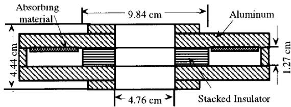
Figure 1. Illustration of the test pillbox cavity.
