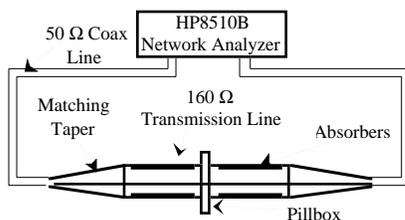
Figure 2. Impedance measurement setup.
