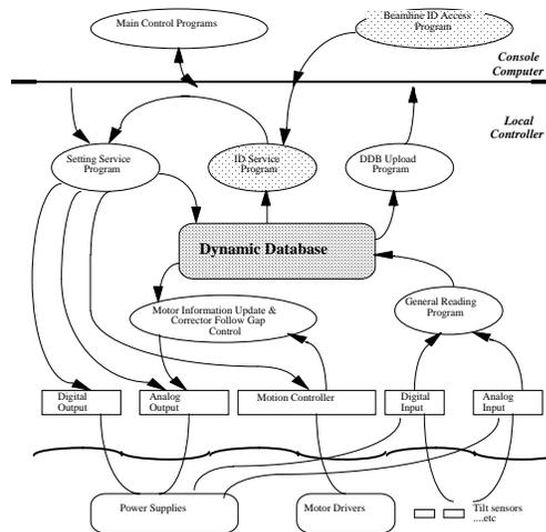
Figure: 1 Software structure on U10P controller
