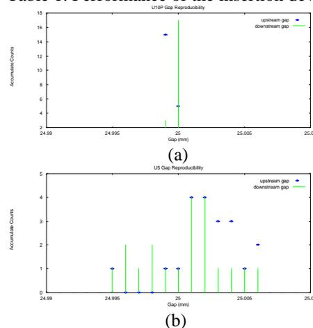
Figure: 2 Gap setting from different gap position to 25 mm (a) reproducibility of the U10P (b) reproducibility of the U5
