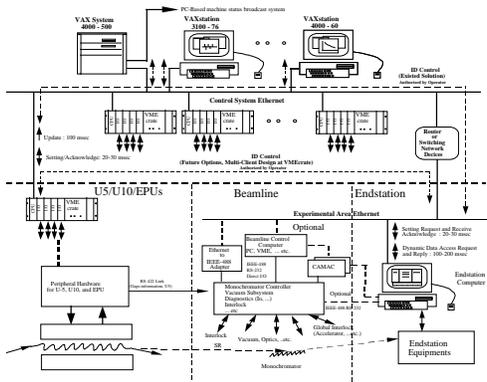
Figure: 4 Relation between main control system, U10P controller and the beamline end-station
