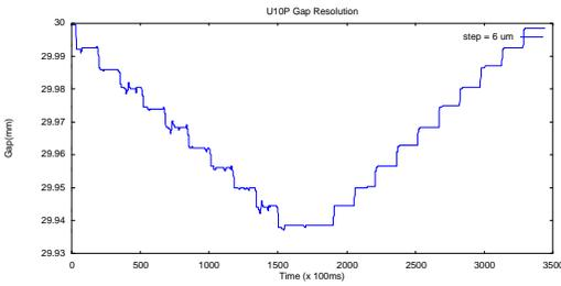
Figure: 5 Simulate beamline request gap change scenario for U10P
