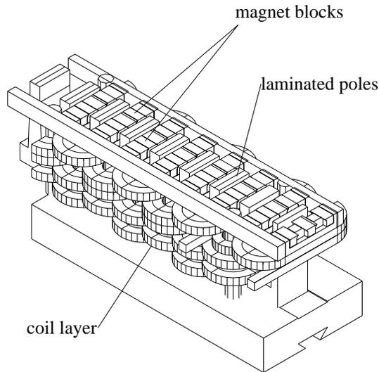
Figure 4: Design of the central part and termination of a novel type permanent -magnet / electro-magnet variable polarisation helical undulator.
