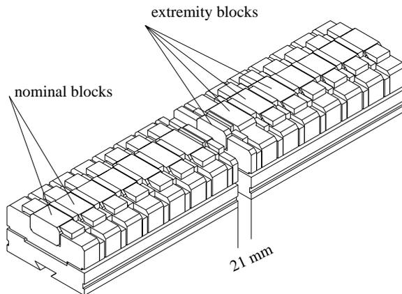
Figure3: Phasing section for an Hybrid Undulator. Due to the large interaction between magnet arrays, the distance between the arrays is increased to 21 mm resulting in some variations of the phase as a function of the magnetic gap.
