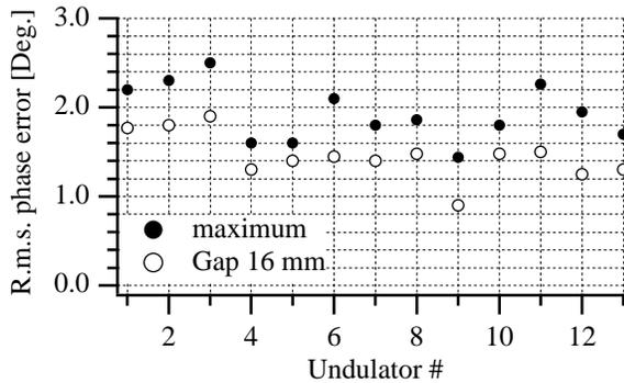
Figure1: rms phase error of the last 13 Undulators produced at ESRF.
