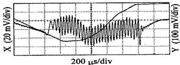
Figure 3. X and Y trajectories from pulsed wire.
