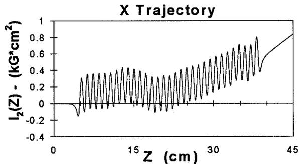
Figure 1. IVUN on-axis trajectory at 3.3 mm gap.
