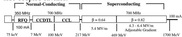
Figure 1. APT Accelerator Schematic.
