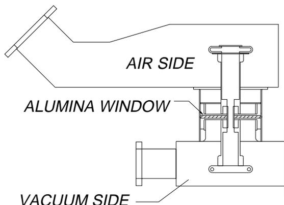
Figure 5. 350 MHz RF coaxial window.
