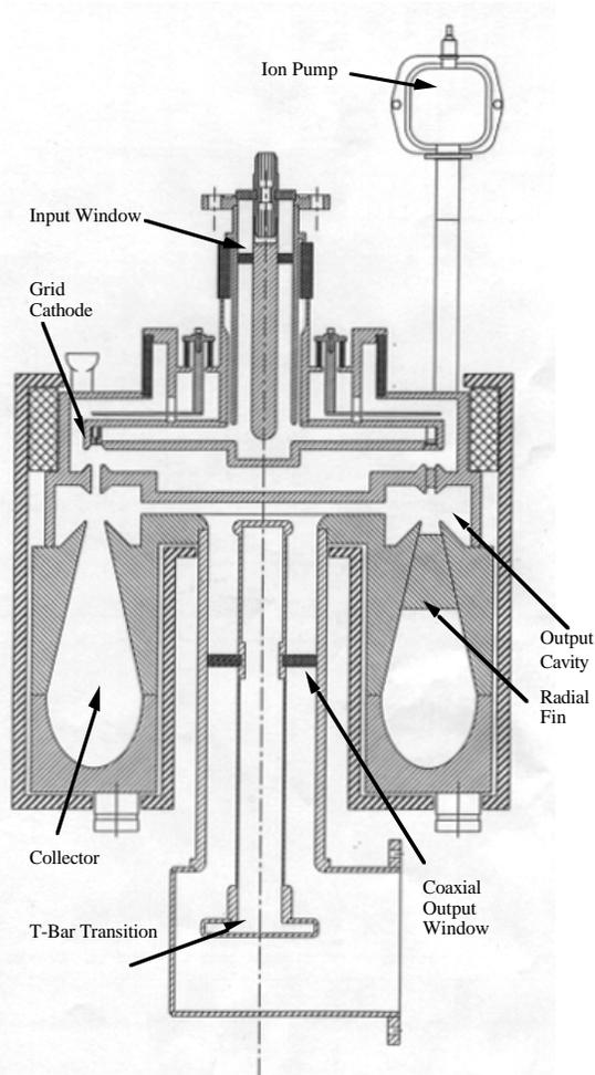
Figure 3. Cross-sectional view of HOM-IOT.
