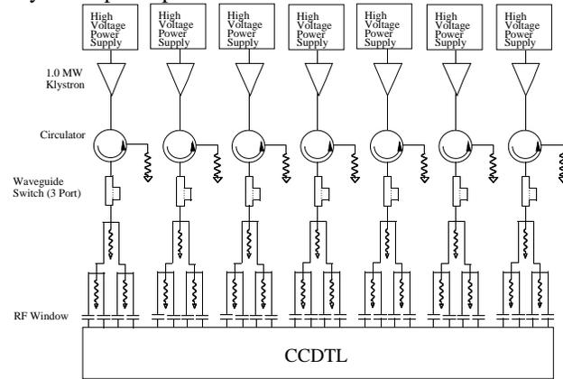
Figure 2. RF Supermodule
