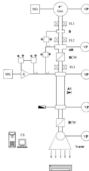
The injector is designed to inject a well-bunched ( $20^\circ$ ), well-collimated and sufficiently accelerated ( $E > 300$  keV) beam of electrons into the accelerator section. The injector consists of an electron gun, a prebuncher (B), an accelerating resonator (AR) and two magnetic thin lenses (FL1 and FL2). The electron gun which operates at  $\sim 25$  kV is of diode type with oxide cathode  $\varnothing 15$  mm.
