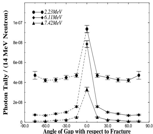
Figure 3. Calculated angular response to a 1 mm fracture in dry granite, filled with water containing 0.3 g/cc NaCl. Photon yields are normalized to the response at 0 degrees (collimator aligned with fracture).
