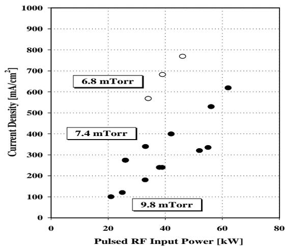
Figure 1. Peak extractable current density at three different source pressures, versus rf input power.
