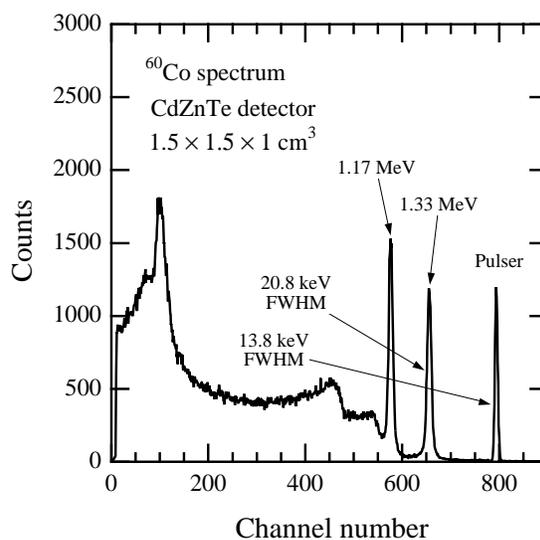
Figure 2. Spectrum of <sup>60</sup>Co obtained using a coplanar-grid CdZnTe detector operated at a temperature of approximately -10°C and at a detector bias of 1600 V.
