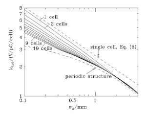
Figure 3: The loss factor  $k_{tot}(\sigma_z)$  obtained by MAFIA for a Gaussian bunch in a structure consisting of a finite number of cells (1-10) Also shown are the single cell (Eq. 6) and the periodic structure loss factor.
