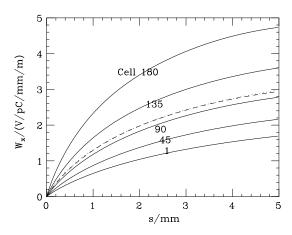
Figure 2: The transverse (dipole) wakefield of representative cells in the SBLC structure (solid curves). The dashes give the average, the dots the model fit, Eq. 5.
