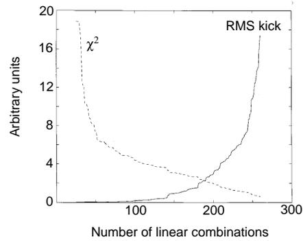
Figure 4: The  $\chi^2$  and the RMS kick found by SVD as a function of the number of linear combinations that are included into the solution. The  $\chi^2$  can be greatly reduced with just a few kick combinations. If too many combinations are included, unphysically strong kicks are introduced that reduce the  $\chi^2$  only slightly.
