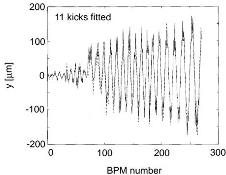
Figure 3: Measured change  $\Delta y_2$  in the electron trajectory due to moving the electron bunch 1 RF bucket (10.5 cm) closer to the positrons. The measurement (solid) is compared to a fit (dashed) for 10 wakefield deflections and an average offset of all structures (compare next section).
