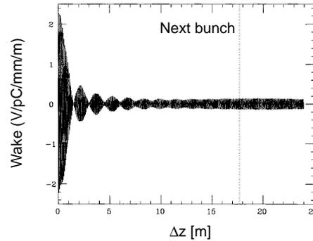
Figure 1: Transverse wakefield as a function of distance  $\Delta z$  for the SLC S-Band structures. The nominal bunch spacing is indicated by the dotted line.
