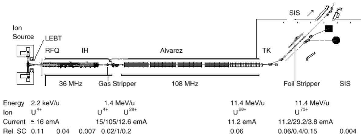
Figure 1: Unilac plan view and high current beam parameters (SC: space charge force)
