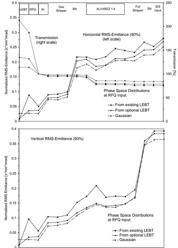
Figure: 2 Transverse rms emittances along the UNILAC for different input beams; Transmission (normalized to 100% at the RFQ exit)
