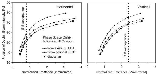
Figure: 3 Beam intensity within partial transverse emittance at injection into the SIS. Intensity is normalized to the design current of 3.8mA  $U^{73+}$
