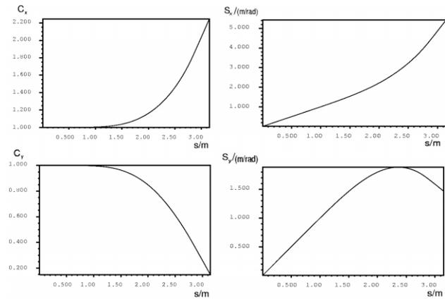
Figure 9: Principal trajectories of the ESR injection line.
