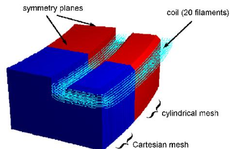
Figure 3: Approximated part of the dipole which is used for the field calculation.
