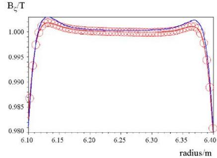
Figure 5: Simulated and measured magnetic flux density at the magnetic mid plane.
