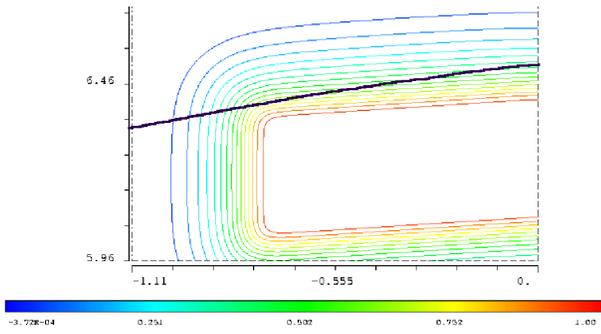
Figure 6: Magnetic flux density at the mid plane with calculated reference trajectory.
