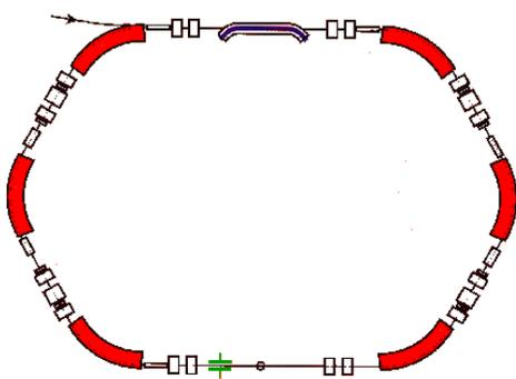
Figure 1: Layout of the ESR with injection line.
