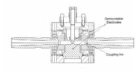
Fig. 4. TM<sub>020</sub> RF breakdown test cavity assembly
