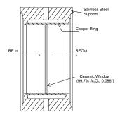
Fig. 5. Output ceramic window.
