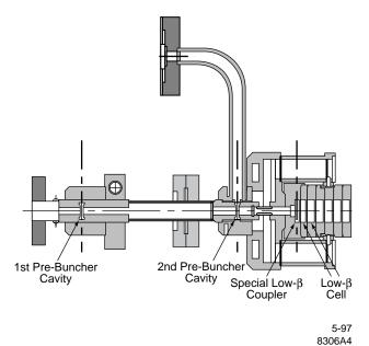
Figure 2: Prebunchers and Front End of 1st 0.9 m Accelerator Section.
