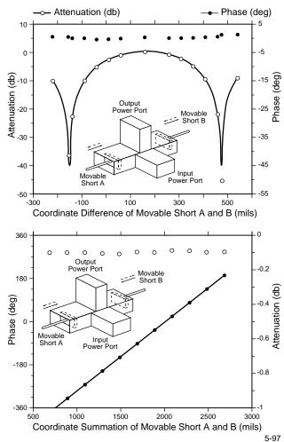
Figure 3: Calibration curves for Magic-T Type Phase Shifter and Attenuator.
