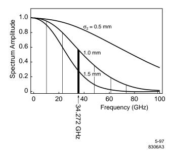
Figure 4: Theoretical Beam Power Spectra for Three Different Bunch Distributions.
