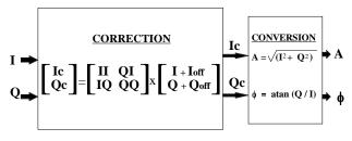
Figure 3. Software algorithm for the I/Q Demodulators
