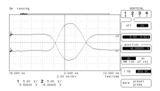
Figure 3: High voltage pulse at both outputs (attenuation 1:120).
