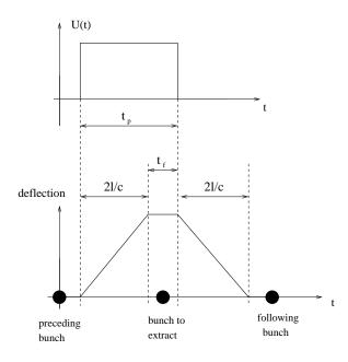
Figure 2: Operation of traveling wave kicker.
