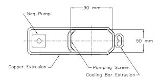
Figure 3. Cross-section of the LEB IR Chamber
