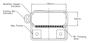
Figure 1. Cross-section of the HEB IR Chamber
