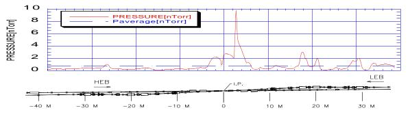
Figure 5. Interaction Region Plan and Pressure Profile
