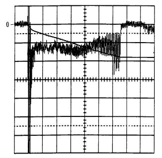
Fig. 2 Extraction of a single pulse from the ring. The vertical scale is 4.2  $\mu$ a/div, and increasing current is down on the graph. The horizontal scale is 0.2 ms/div. Also shown is the integral of the extracted current.
