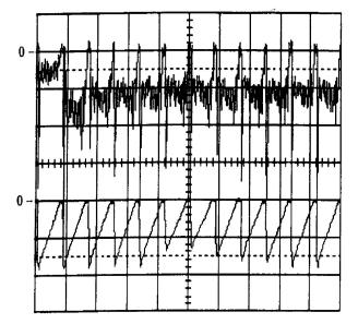
Fig.3 Extraction of a train of pulses injected into the ring at 600 Hz. The upper trace is the extracted current, and the lower trace is the current in the ring. For both traces, increasing current is down. The horizontal scale is 2 ms/div. The average extracted current is a few microamps.
