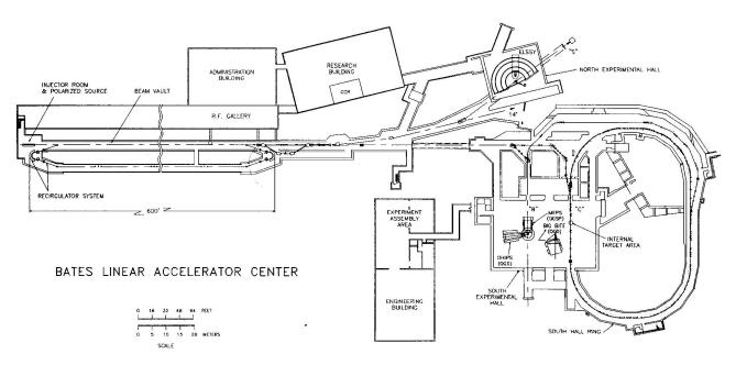
Fig. 1 Layout of the Bates facility, including the South Hall Ring and associated beamlines
