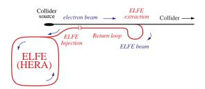
Figure 1: ELFE@DESY schematic layout
