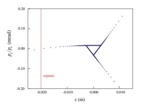
Figure 2: Separatrix triangle (with ELFE@DESY parameters)
