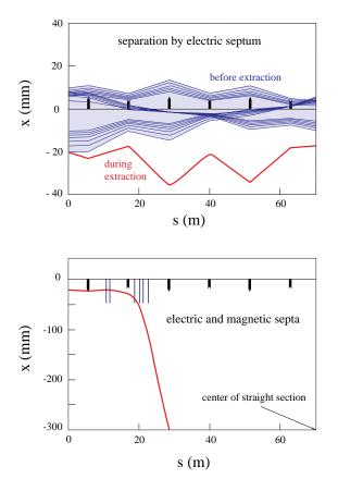
Figure 4: Extraction channel
