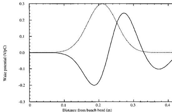
Figure 6: Wake potential of injection kicker
