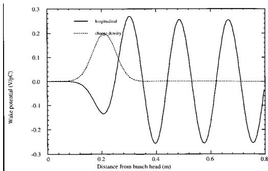
Figure 5: Wake potential of bellow gaps
