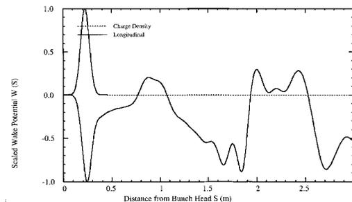
Figure 2: Wake potential of BEPC cavity
