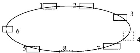
1-RF cavities, 2-Separators, 3-kickers, 4-Bellow gaps
