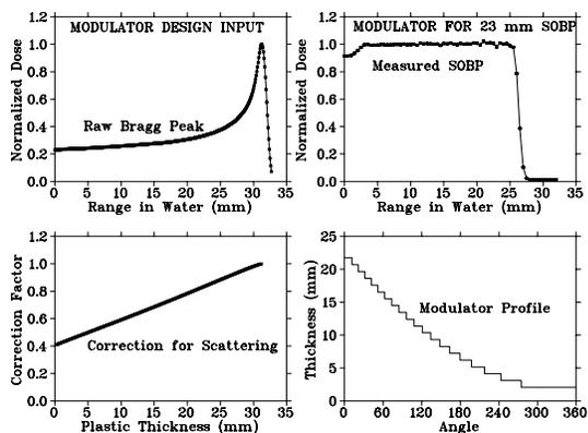
Figure 3: Input data for the modulator design and a measured result.
