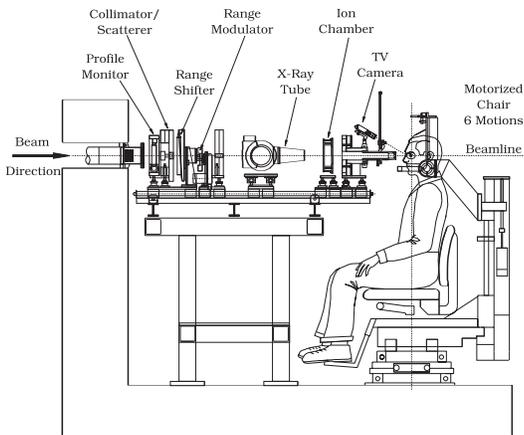
Figure 2: Arrangement of the equipment for beam delivery and patient fixation.
