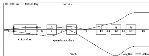
Figure 5: Beam envelopes of the high energy beam transport line.
