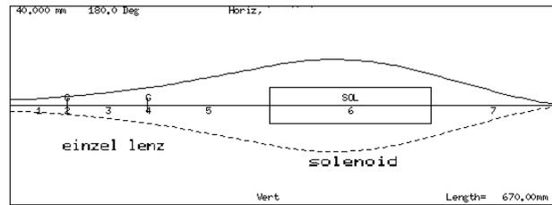
Figure 4: Beam envelopes of the low energy beam transport line.
