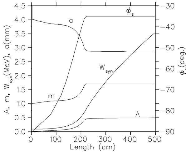
Figure 2: Cell parameters of the RFQ as a function of longitudinal position
