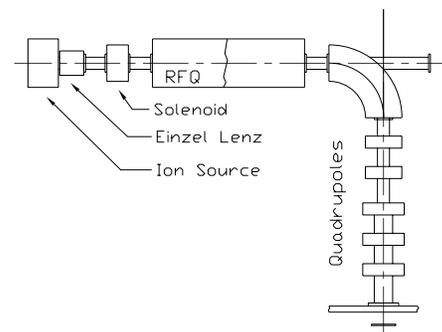
Figure 1: A schematic view of a linear accelerator system for BNCT
