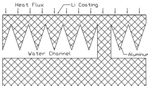
Figure 6: A preliminary design of a Li target.
