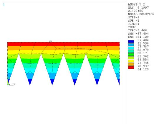
Figure 7: Temperature distribution on the Li target calculated with ANSYS. See text for details.
