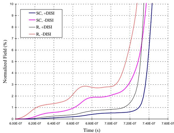
**Figure 3. Pre-pulse kicker field with 80kV PFN, DS and MS DISI, with and without a 12cm<sup>2</sup> DISI, with a short-circuit terminator or a resistive terminator.**
