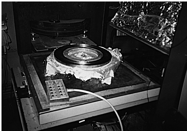
Figure: 2 The furnace for cores with OD up to 700mm.
