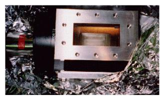
Figure 3: Vendor 2's WR-340 waveguide switch.
