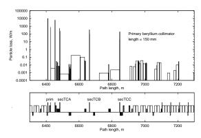
Figure 1: Beam loss distribution in the IP3 beam collimation region at collisions for 150 mm beryllium primary collimator.
