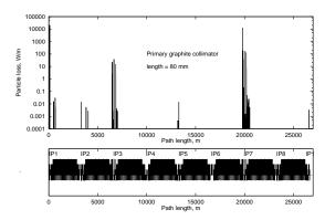
Figure 2: Beam loss distribution in the LHC lattice at momentum cleaning for a 80 mm graphite primary cillimator in IP7.
