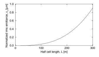
Figure 1: Equilibrium emittance versus half cell length
