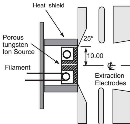
Figure: 1 Schematic diagram of the ion source and extraction electrodes.
