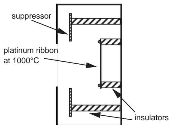
Figure: 2 Schematic diagram of the neutral detector
