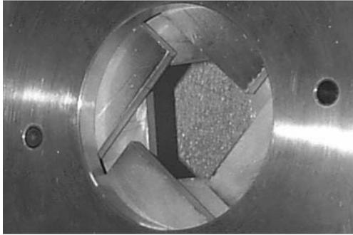
Figure 4. Beam iris developed for the LEDA LEBT.
