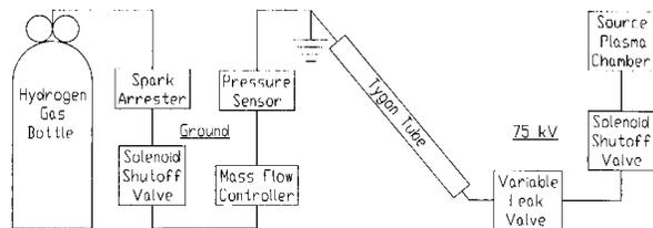
Figure 3. Gas flow control for the LEDA ion source.
