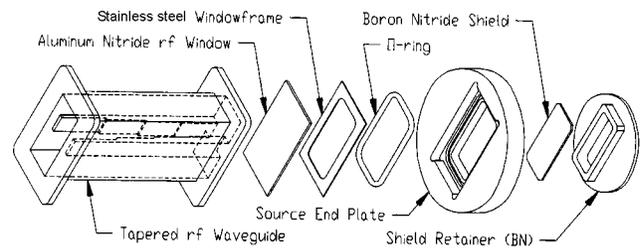
Figure 2. LEDA proton source microwave window.
