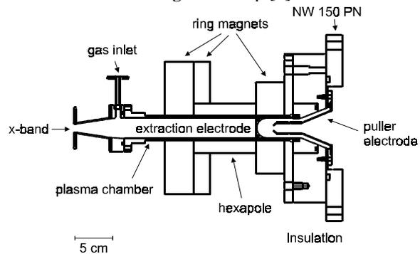
Fig. 1: Schematic view of the 10 GHz ECRIS
