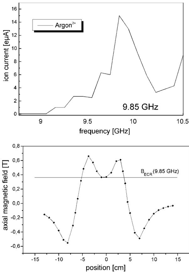
Fig. 2: Frequency dependence of the extracted Ar 2+ beam intensity with corresponding axial magnetic field using another permanent magnet configuration with a mirror ratios of 2.5 and 1.6, respectively. The best results were obtained at a frequency of 8.85 GHz, for which the resonance field was close to the minimum of the magnetic mirror.
