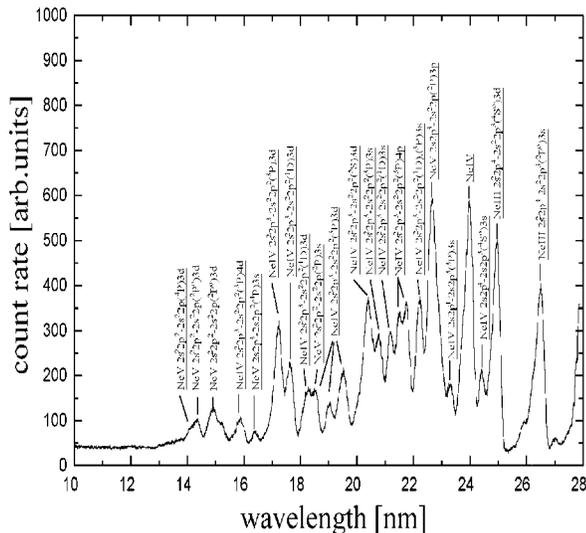
Fig. 3: Detailed line spectrum obtained from a Ne plasma using a 32cm grazing incidence spectrometer
