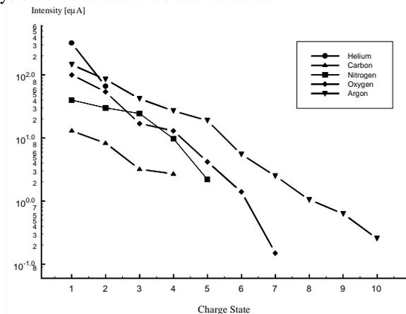
Fig. 4: Beam intensities for various gases at an extraction voltage of 9 kV.
