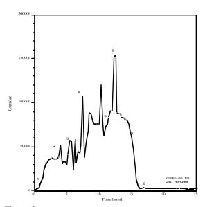
Figure 3 1.Insertion device gaps open 2.Ramp 1.5 to 1.9 GeV 3.Injection process begins 4.Beam stacking
