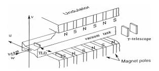
Figure 1: ALS insertion device showing coordinate system, vacuum tank, TLD and γ-telescope
