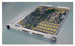
Figure 1. VXI Fast Interlock Module
